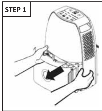
Slide water tank out
